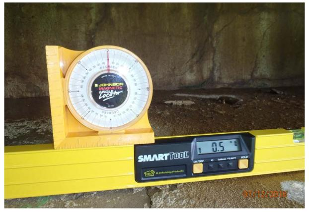
Close-up the smart level reading taken between beams 1 and 2 at abutment 6.
