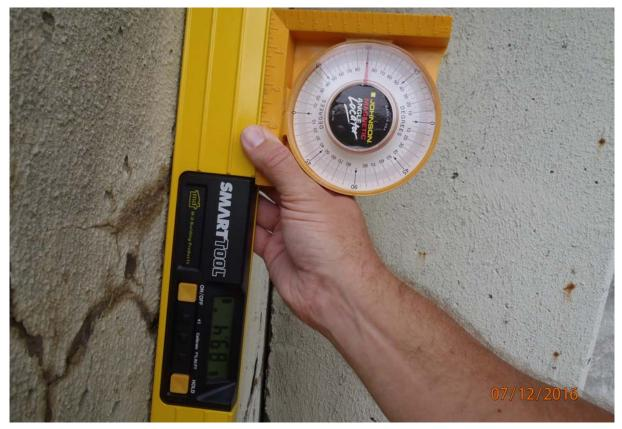
View of the level reading taken at the above location. Note when the smart level was flipped the reading did not change; this smart level is assigned to B. Jones and the calibration might vary slightly.
